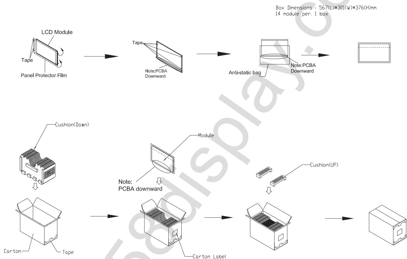
**Figure. 8-1 Packing method**
