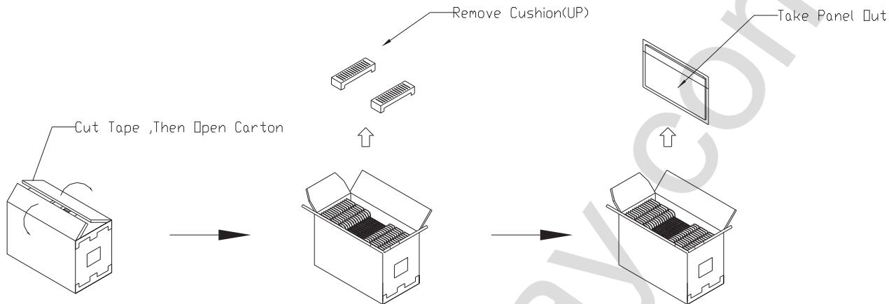
Figure. 8-3 Un-packing method
